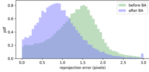
Figure 4. Distribution of reprojection errors before and after bundle adjustment, site 1.
